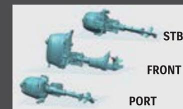
The design allows the outboard to be removed from the boat and placed on 3 sides for storage.
