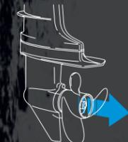
**Propeller hub exhaust**
