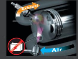
**Battery-less electronic fuel injection**
